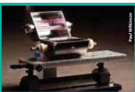
This laser was developed in the USA in 1964, and was one of the first to come into the UK when George Porter, director of the Ri, bought it. Known as a ruby laser, it was used to speed up chemical reactions with short bursts of energy
