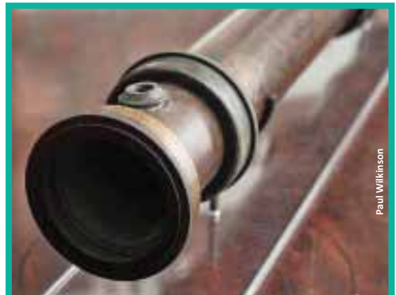
This object from 1859 has had a huge influence on our understanding of climate change. It's a tube used by Irish scientist John Tyndall to measure whether gases absorbed or transmitted heat in our atmosphere. Tyndall's experiments discovered greenhouse gases and their effects on our planet – the basis of climate change
