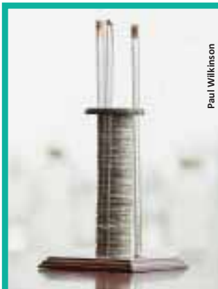
Dating back to the start of the 19th century, this is one of the first electrical batteries. It was invented by Italian scientist Alessandro Volta and was given to Michael Faraday in 1814
